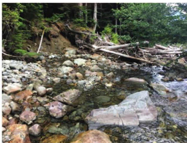
South Fork Sauk River arsenic monitoring site. The braided stream makes flow difficult to measure, which adds uncertainty to arsenic results here. 9
