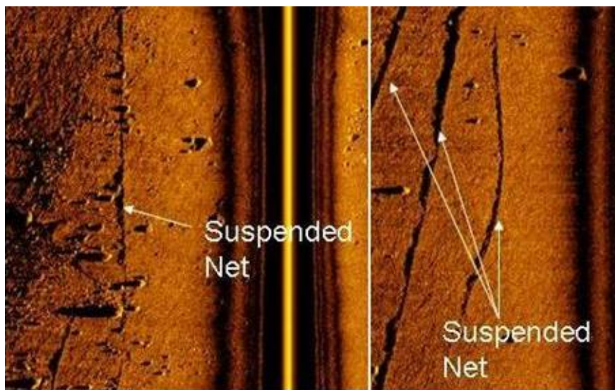
Figure 13. Sidescan sonar images of deepwater derelict nets located on Point Roberts Reef of the San Juan basin. Suspended nets have a larger acoustic shadow than nets flush with the bottom. Image courtesy of Natural Resource Consultants.
