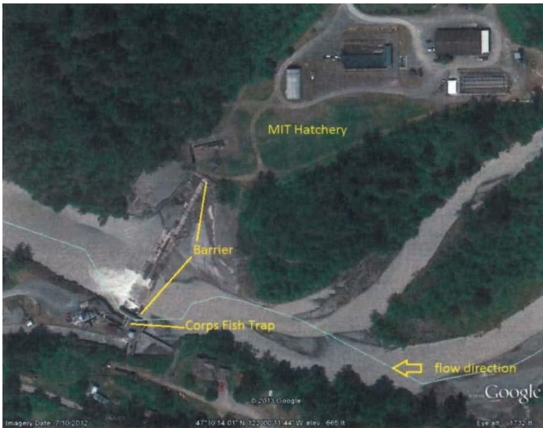
Figure 1 Aerial view depicting White River diversion dam (barrier), the Corps' fish trap, and the Muckleshoot Indian Tribe's White River hatchery
