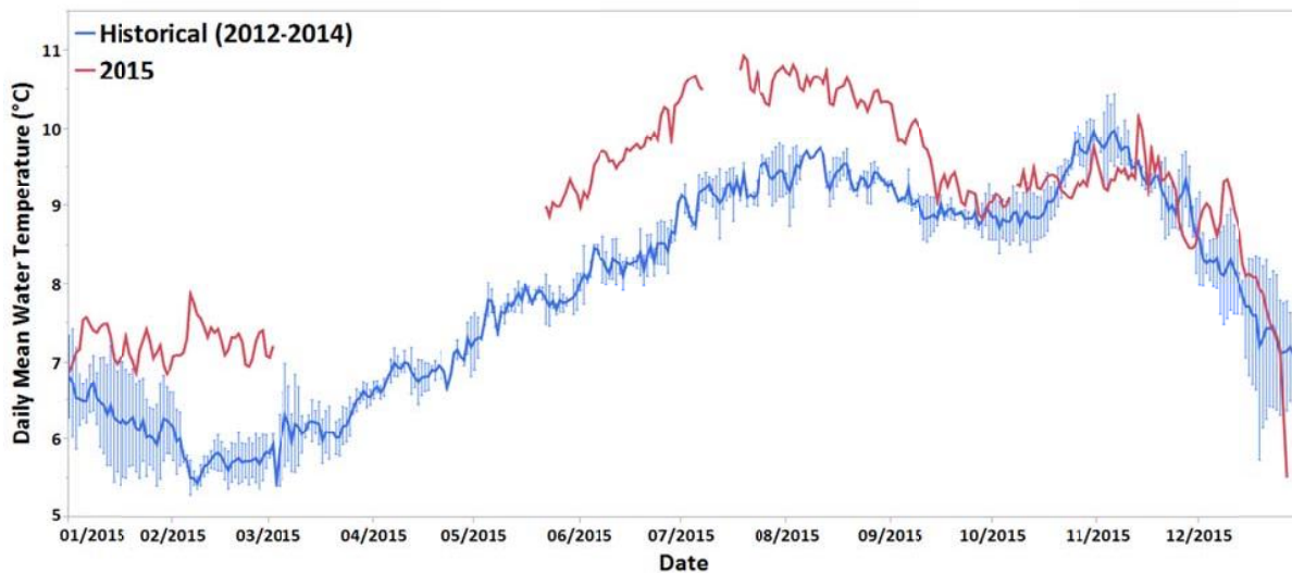
Figure 4-15. Historical (2012 through 2014) and 2015 daily mean water temperatures at the compliance point (RM 13.3) in the lower North Fork. Blue bars represent the historical range of mean daily flows. From Tacoma Power (2016).
