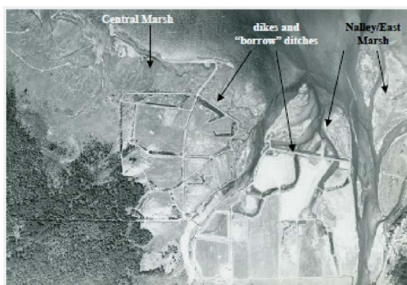
Figure 4.46. A 1958 air photo showing the system of dikes and borrow ditches and pits, most of which was constructed between 1938 and 1942. From Todd et al. (2006).
