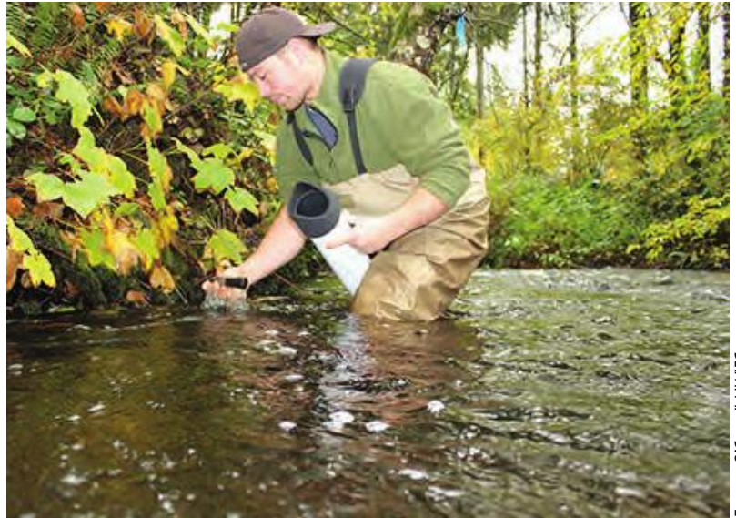
Joe Puhn, natural resources technician for the Squaxin Island Tribe, takes a velocity measurement on Goldsborough Creek.
